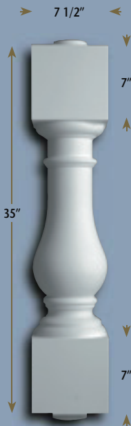
BAL 2212-35 • 1 1/2" "M" Dimension • 7/8" Max. Space 4" Ball Rule • 1 13/16" Hole Saw
