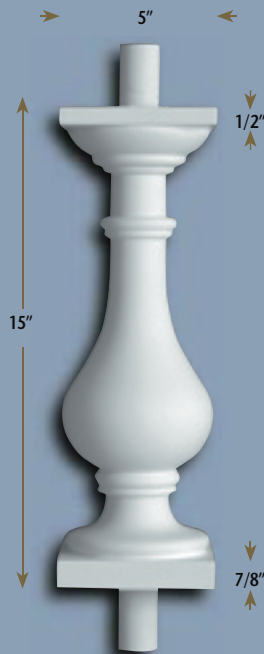
BAL 2090-15 • 1 5/8" "M" Dimension • 1 1/16" Max. Space • 4" Ball Rule • 1 3/4" Hole Saw
