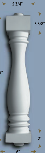
BAL 2245-29 • 1 17/32" "M" Dimension • 13/16" Max. Space 4" Ball Rule • 2 9/16" Hole Saw
