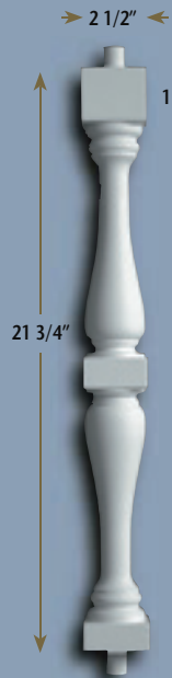
BAL 2240-28 • 7/8" "M" Dimension • 2 1/8" Max. Space 4" Ball Rule • 3 1/16" Hole Saw
