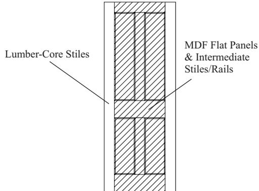
**NEWPORT:** The "Newport" collection includes a series of door styles that are constructed with flat (recessed) plywood panels and lumber core stiles/rails. Newport doors are available in both 1 3/8" and 1 3/4" thicknesses.
